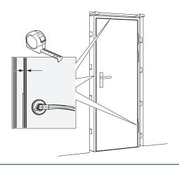
Final undercut from bottom of the door to finished floor level must not exceed 6 mm. Doors with smoke seal must not exceed 3 mm from bottom of door to finished floor level. Finished floor must be of noncombustible material.
