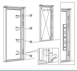
Install the striker jamb, starting with the bottom screw first.
