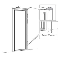
Adjust the frame till the frame top is plumb.
