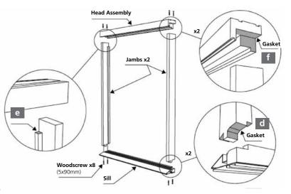
Check the corners of the frame are square and the diagonals of the frame are within 5mm of each other. If not loosen screws adjust and re-tighten.
