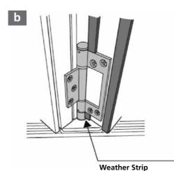
Adjust the top and bottom pivot hinges to ensure the door is vertical and set 5mm from the top track.
