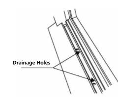
Check once more, that the jambs are vertical, that the head and sill are level and that the diagonals are within 5mm of each other.
