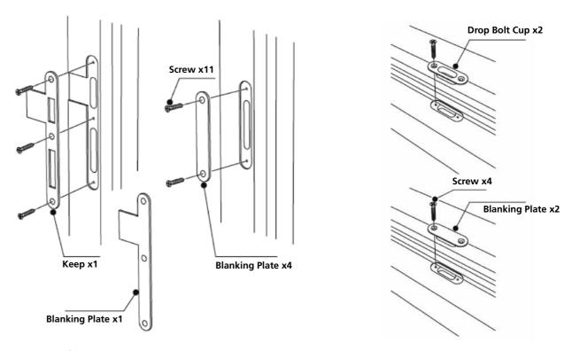
The recess for the centre keep in the door is intentionally larger than the keep in order to be reversible.
