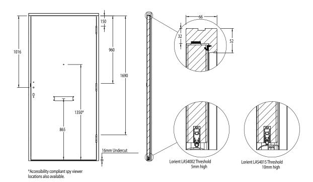
Dimensions shown on drawing detail the default hardware locations, based on standard sized flush doors. Dimensions will vary slight on Made to Measure products and moulded options to suit the design of the doorset.
