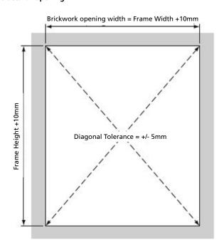
**Note:** To calculate the overall frame width for a doorset with winglights or dwarf winglights simply add the actual frame dimensions for each component together across the width.
