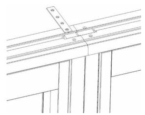
Before coupling together, seal the end grain of both head and sills with suitable end grain sealant. A flexible sealant should then be used the full length of the joint, but with particular attention at the sill joint.
