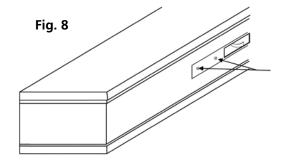
Do not tamper with the two screws directly above the top hook as these hold the reverse gearbox to the Espagnolette. Fig 8
